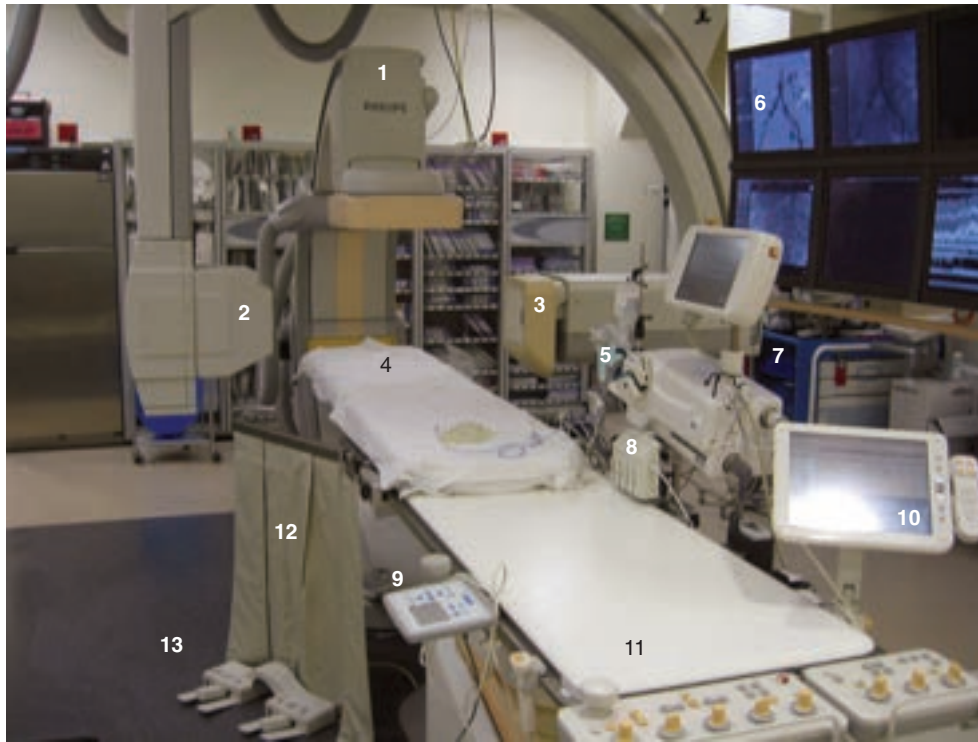
E-FIGURE 57-1. Modern cardiac catheterization laboratory. (1) Anteroposterior imaging gantry. The image intensifier is above the patient and the x-ray tube below. (2) Lateral imaging gantry with the x-ray system to the patient's right and (3) the lateral plane imaging intensifier on the patient's left side. (4) Catheterization laboratory table pad position for patient's head. (5) Power injector for radiographic contrast material. (6) Angiographic and hemodynamic monitor bank. (7) Crash cart. (8) Pressure transducer holders. (9) Monitor displaying intravascular ultrasound image during percutaneous coronary intervention. (10) Control panel for x-ray images. (11) Table controls for movement of x-ray system. (12) Under-table lead shield. (13) Foot pedal controls for fluoroscopy and cineangiography imaging.
